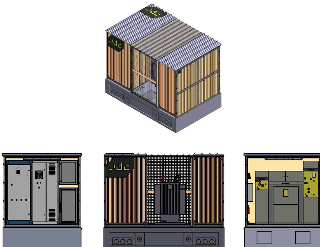
Figure 4 - SKID UPP with Concrete Base Frame
